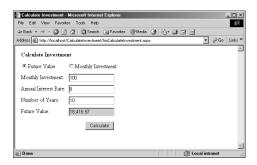
The other type of application is a **Web Forms application**. A web forms application consists of one or more web forms that provide the user interface. A Web Form runs in a web browser.
