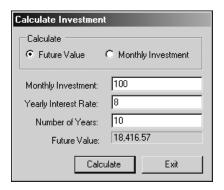
VB.NET is typically used to develop two types of applications. First, is a **Windows Forms application**. A Windows Forms application runs on the user's PC and consists of one or more Windows forms. These forms provide the GUI for the application. Each Windows form can contain controls like labels, text boxes, command buttons, radio buttons, and check boxes, and others.
